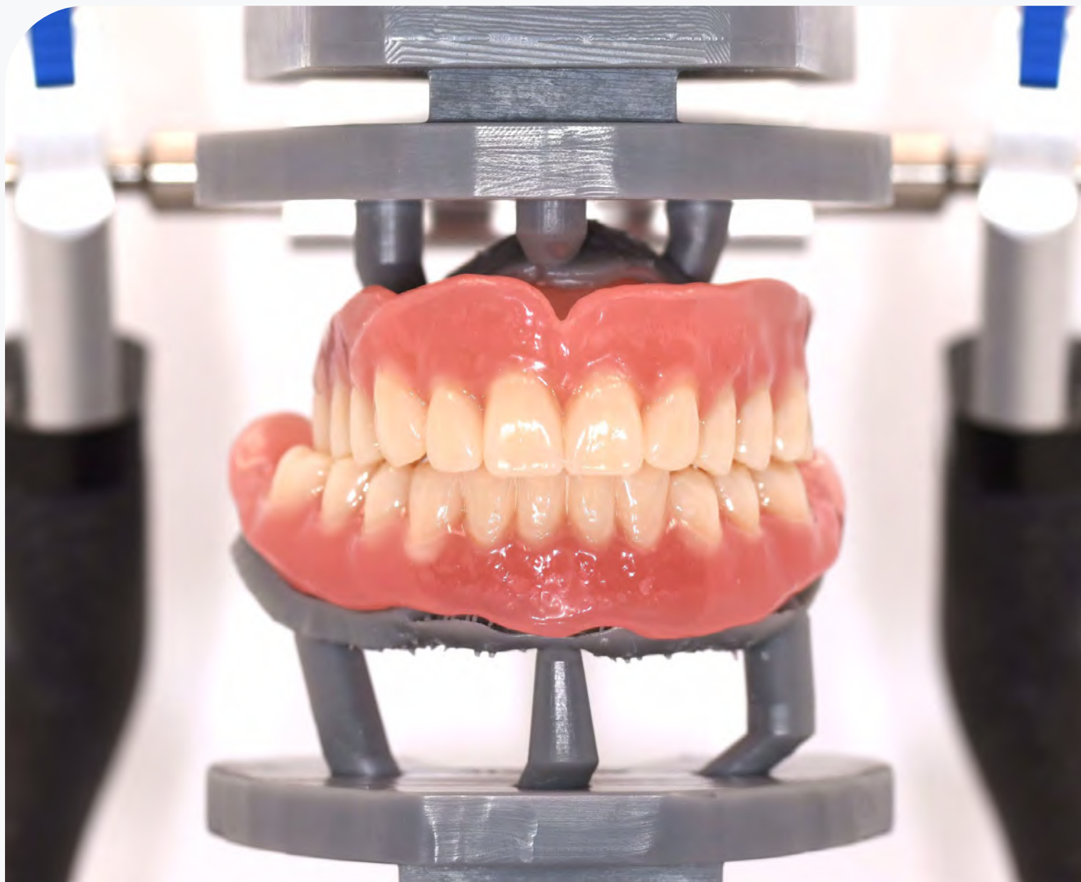
FIG. 23 DACOS system checking of the occlusal contact.
